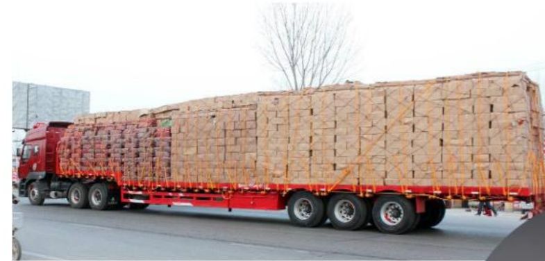
Gooseneck flat low bed semitrailer
