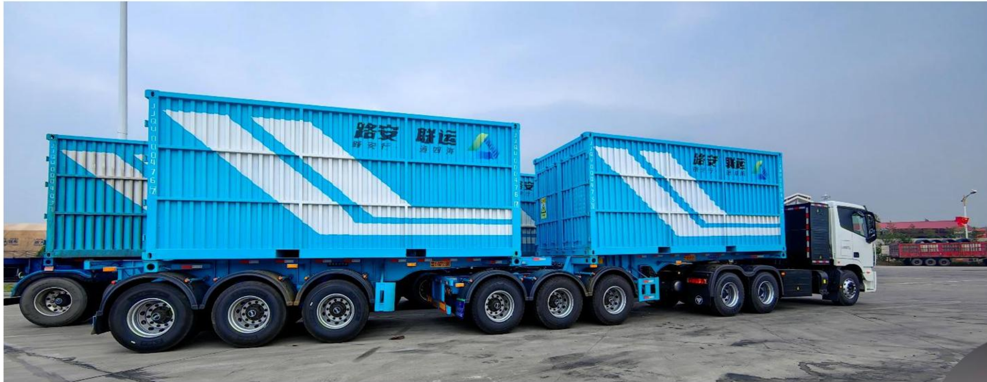
Ordos BEV tractor B-trailer + semitrailer, 45km intermodal Transportation Length: \leq 22.00\text{m} , Weight: \leq 74.00\text{t}
