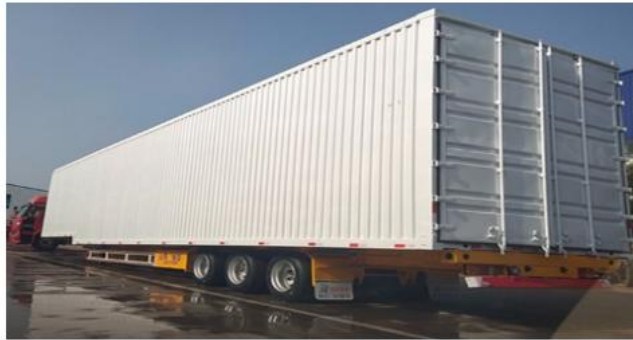
Oversized container box on a compliant semitrailer chassis
