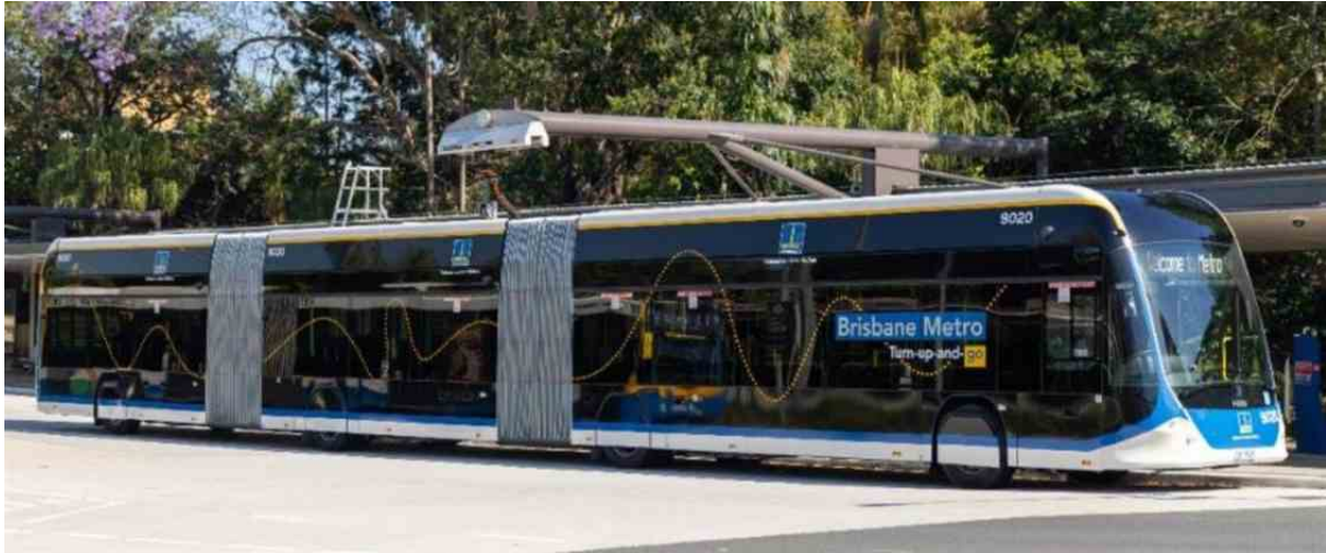
Figure 4. Brisbane Metro “Bus-Up” Pantograph Charging
