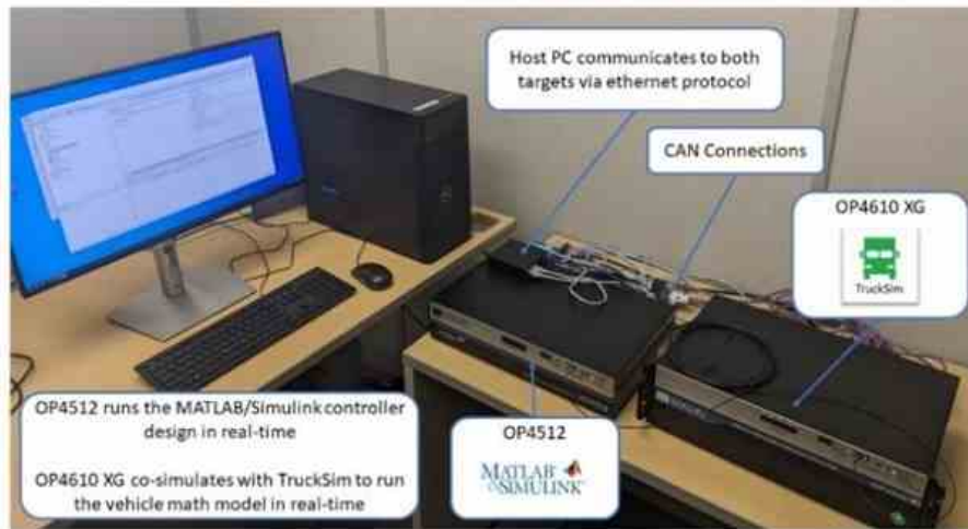
Figure 8 – HIL platform containing the host PC and two real-time target machines.
