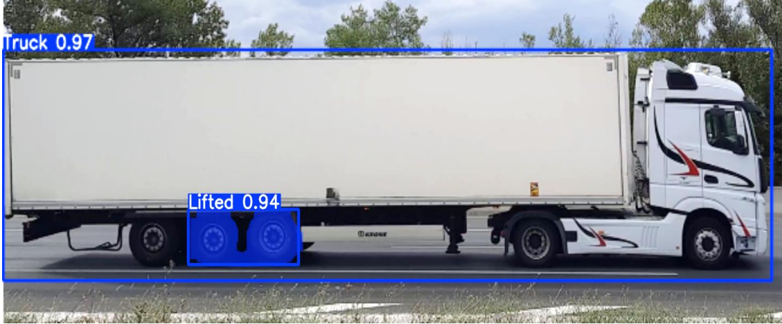
Figure 7 – Example of lifted axle detection by the method
