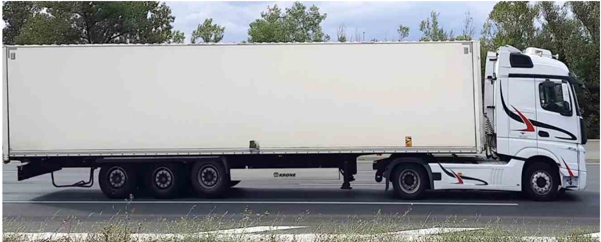
(b) 5-axle truck with 1 lifted axle
