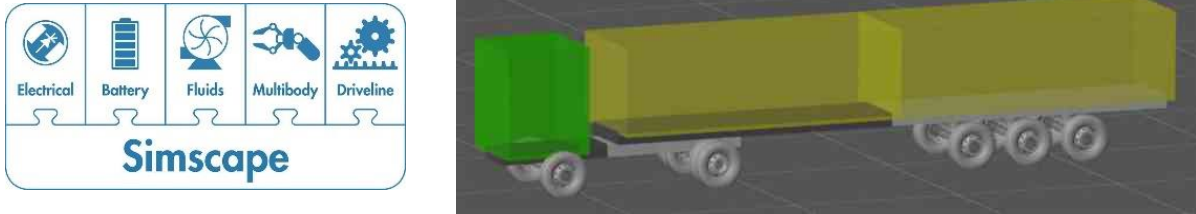
Figure 6 – Tractor Semitrailer multibody model built in Matlab Simscape.
