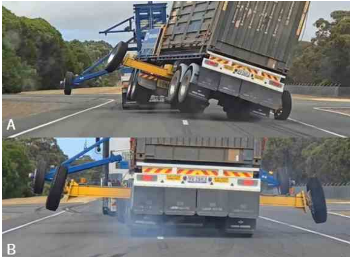
Figure 7 - Test vehicle performing double lane change with RSC off (A) and on (B)
