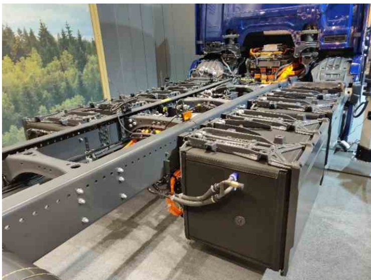
Figure 2. The battery pack used on the truck. Photo by Anton Ahlinder.
