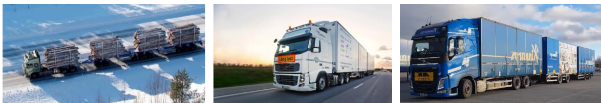
Figure 3 – Examples of tested LVCs in Sweden From left to right: ETT vehicle, DOU-trailer, DUO-CAT
