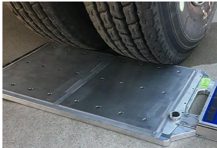
Figure 3 – Measuring Individual Wheel Weights within Dual Tire Configurations
