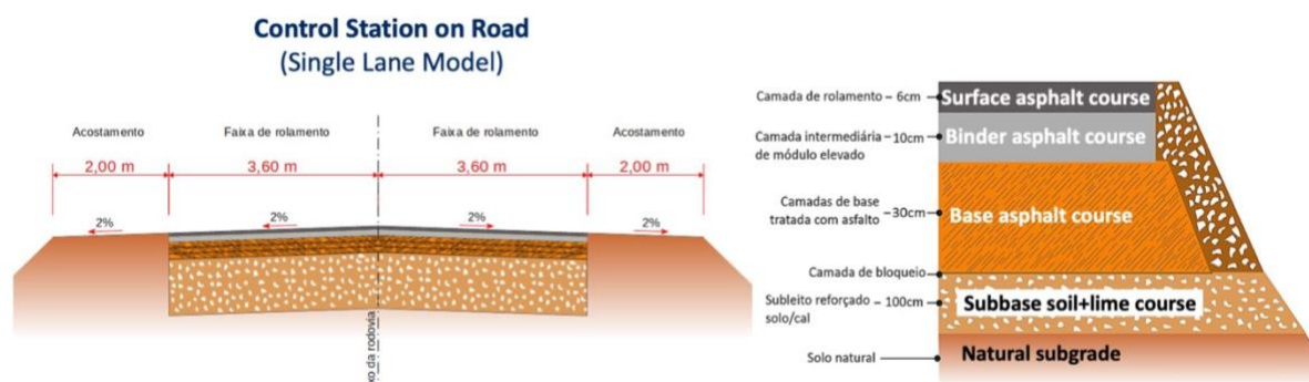
Figure 7 – Thick Asphalt Concrete Pavement (TACP) for HS-WIM system
