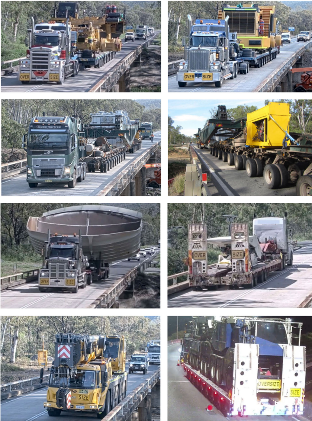
Figure 3 Mobile cranes and combinations incorporating platform trailers and low loaders crossing the Bee Creek bridge and the Gateway Arterial Flyover.
