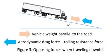
The total calculated forces that oppose to the movement of the vehicle configuration with dry van trailers are the aerodynamic drag force  $(F_d)$  + rolling resistance  $(F_r)$ , and may be expressed in term of power considering the speed of travel of the vehicle as follows:
