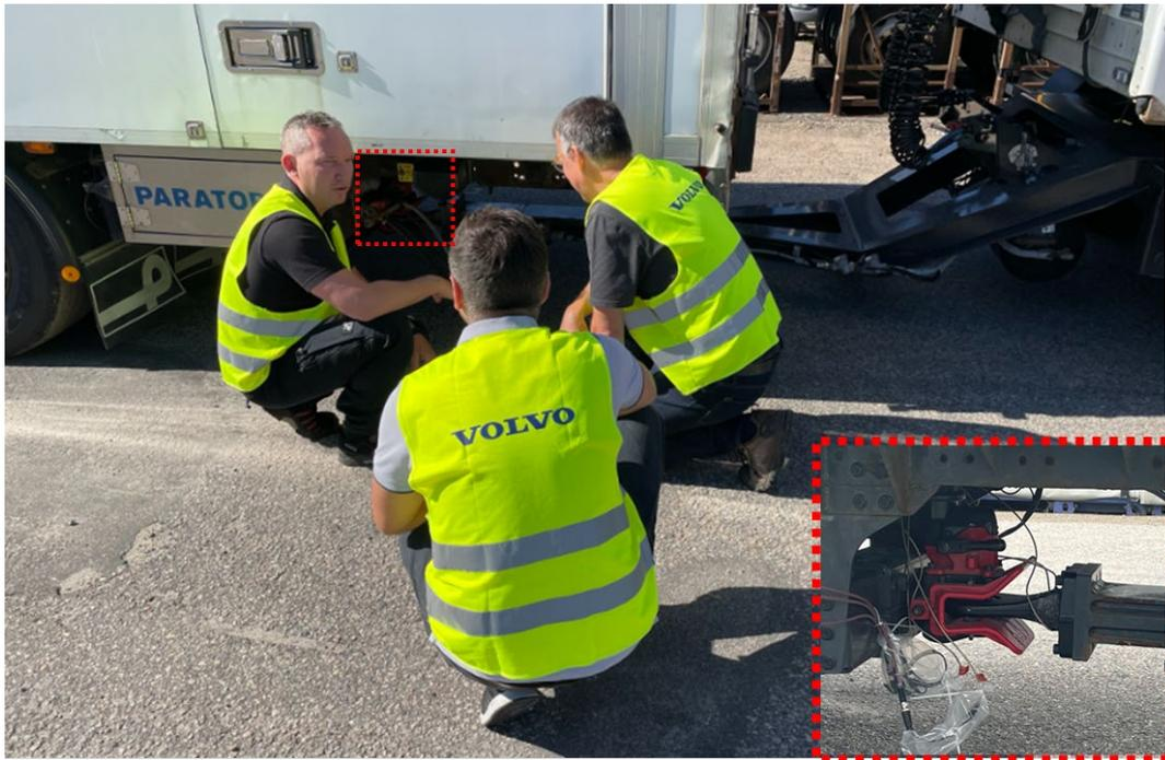
**Figure 3 – Close-up of position of the force sensor on the dolly**
