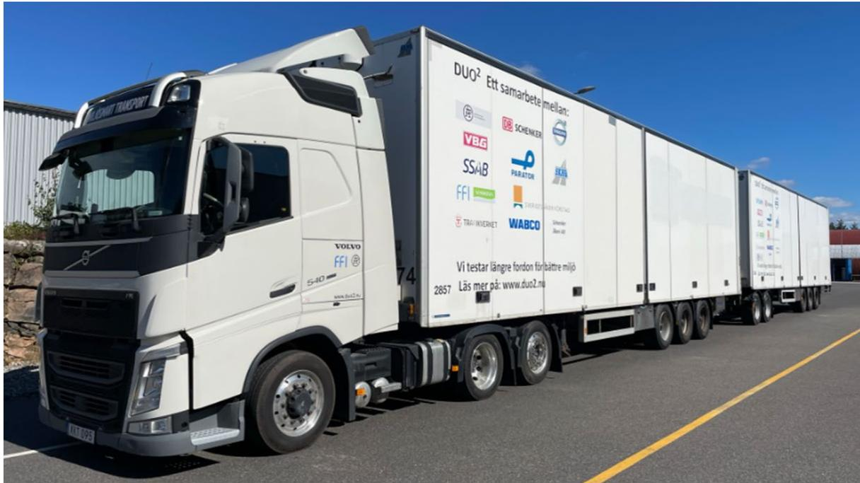
**Figure 1 – A duo-trailer combination with eleven axles, of which five axles are liftable**
