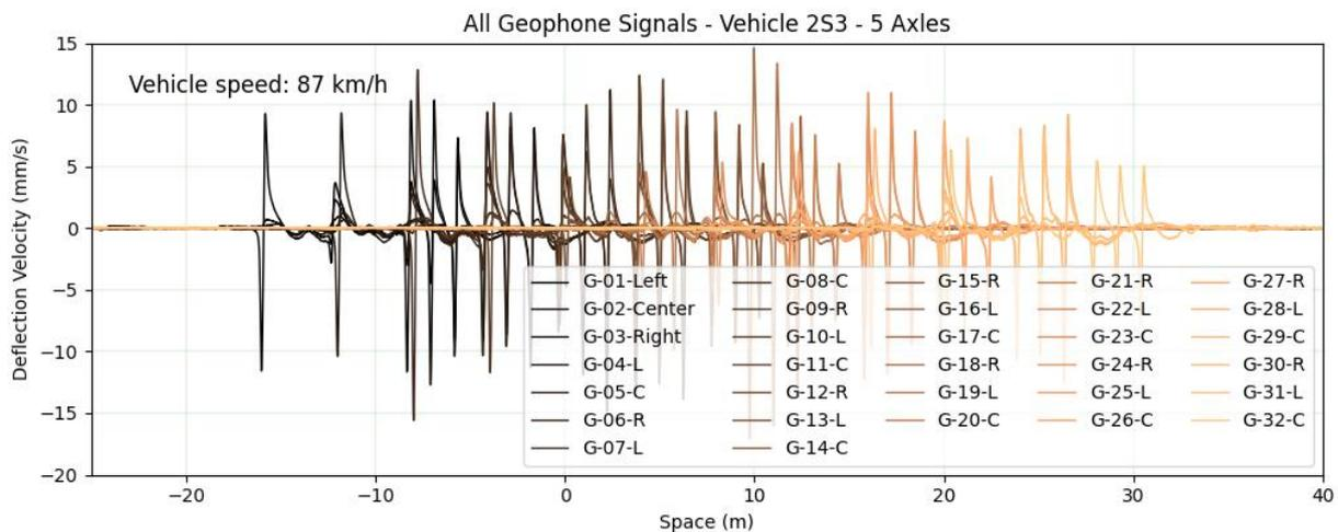
Figure 5 –Singnals from all geophone sensors of the five-axes
