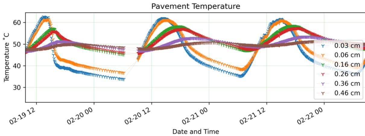
**Figure 2 – Temperature variation on the pavement structure during a period of three days**
