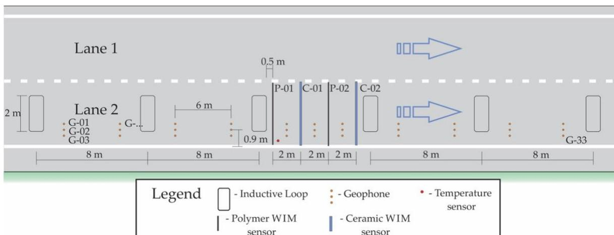
**Figure 1 – Experimental site instrumentation design with WIM system and the groups of geophones**
