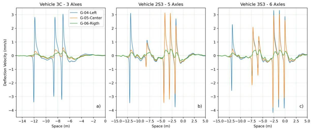
**Figure 5 – Geophone signals (G-04, G-05 and G-06) a) three-axes vehicle, b) five-axes vehicle and c) six-axes vehicle**
