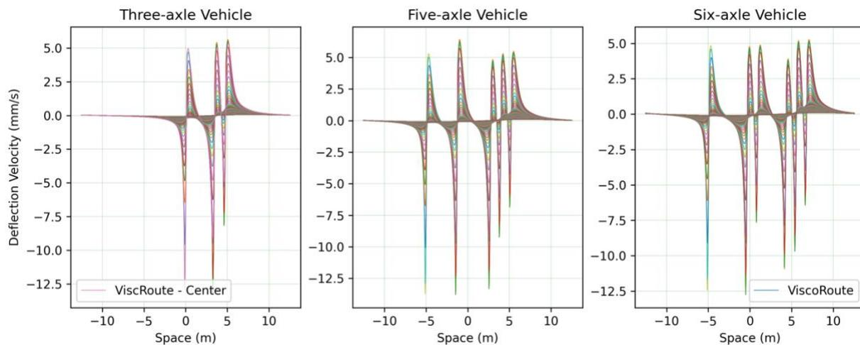
**Figure 2 – Prediction of pavement deflection velocity using the viscoroute mathematical model**
