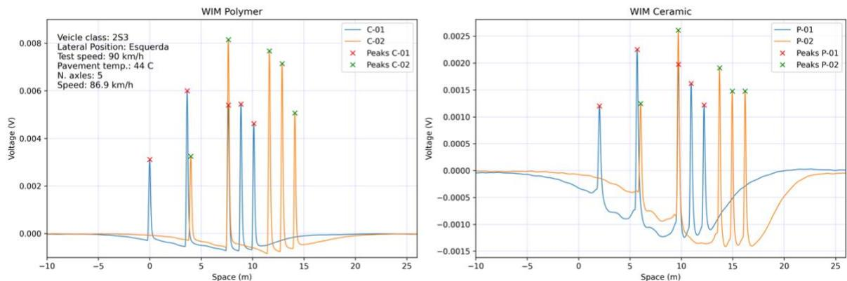
**Figure 3 – WIM sensor electrical response of the 5 axles vehicle, at a position Center, Right and Left a) Polymer (P-01, P02) sensors and b) Ceramic (C-01, C-02)**
