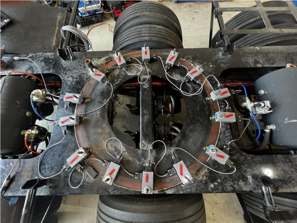
Figure 4 - Layout of the Fifth Wheel Load Sensors
