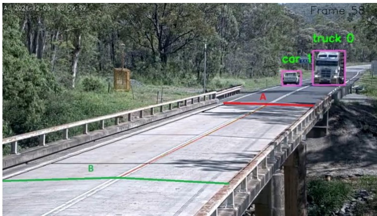
Figure 4.1 - Output of System showing Start A and End B for Speed Estimation
