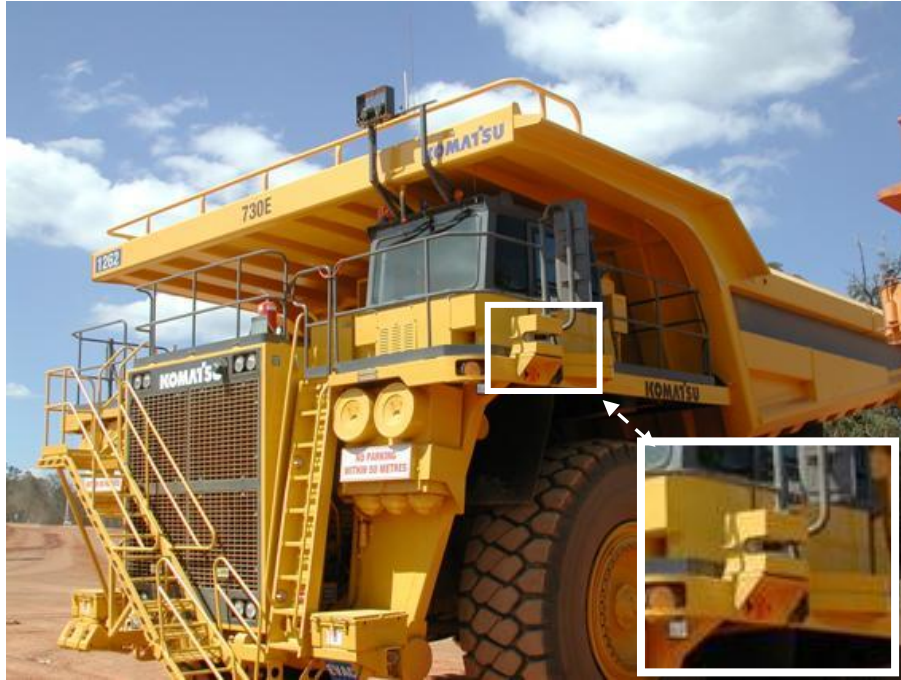
Figure 4: Industrial LiDAR, installed in a truck, laterally” (Truck Guidance System, 2005) (as used in E Nebot, J Guivant (2006) and [E Nebot, J Guivant, S Worrall (2006)
