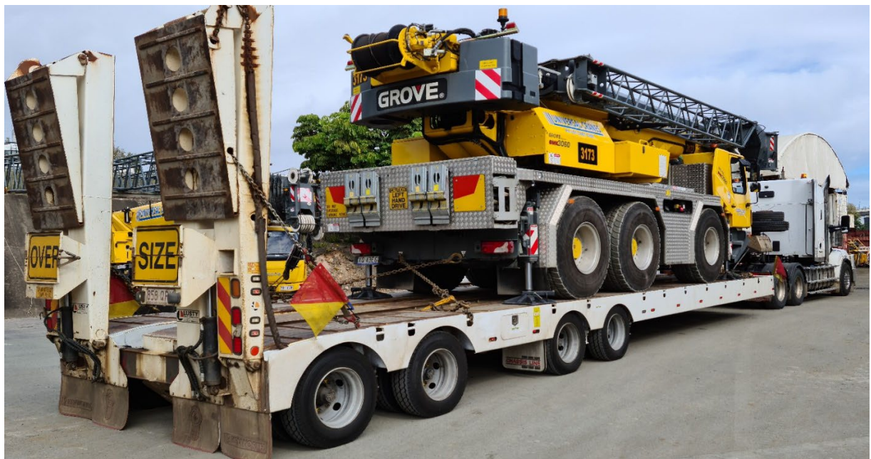
Figure 15 - OSOM Prime mover and Quad Axle low loader (Four Rows of Four) – fully loaded in the depot
