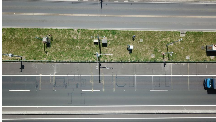
Figure 5 – HS-WIM system test road in Brazil
