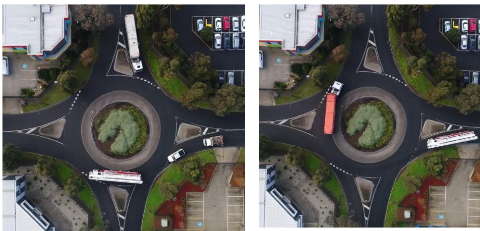
Figure 5 Concrete Pump (left) vs Semi-Trailer (right) on roundabout
