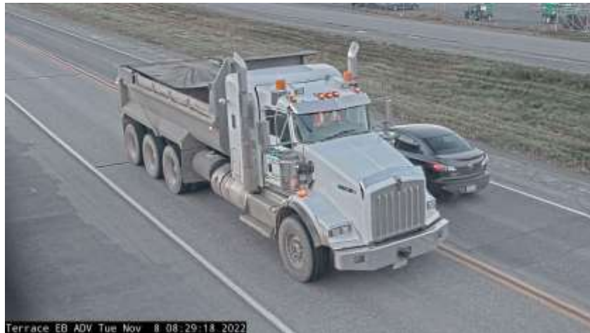
Figure 2 – Typical Commercial Vehicle with Wide-Base Tires on the Steer Axle
