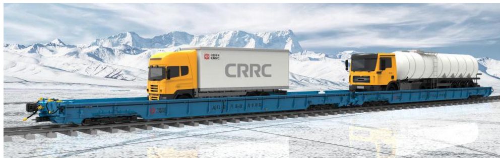
Fig 1 – Small-wheel-diameter and low-floor piggyback transport wagon
