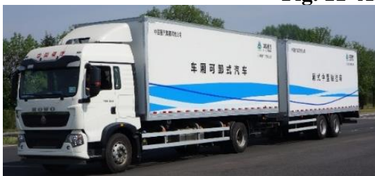
Fig. 13 Centre axle trailer combination
