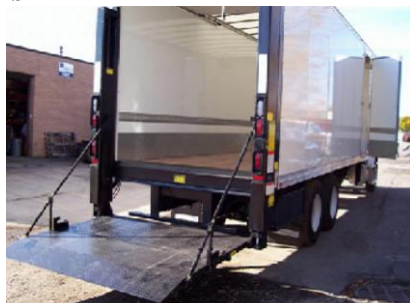
Fig. 7 Hydraulic Ramps for Loading and Unloading
