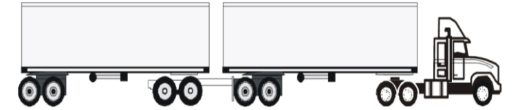
Figure 2 – Typical double trailer configuration T3-S2-R4
