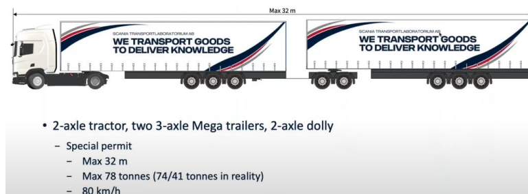
Figure 1: Example of dual trailer system, picture is from Björklund & Sterky
