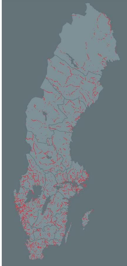
*Figure 4 – Map with the 16 000 unsafe horizontal curves on paved state roads in Sweden*
