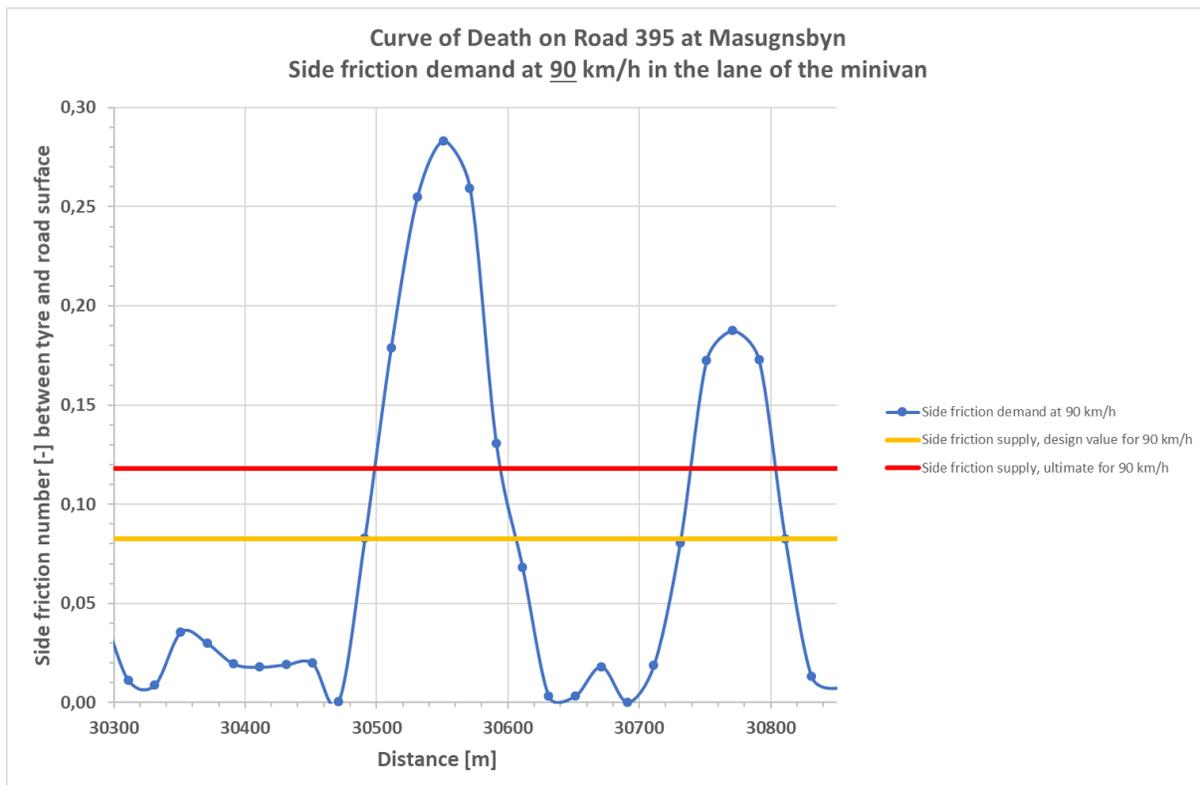
Figure 1 - Side friction demand and supply at the sharp and S-shaped Curve of Death
