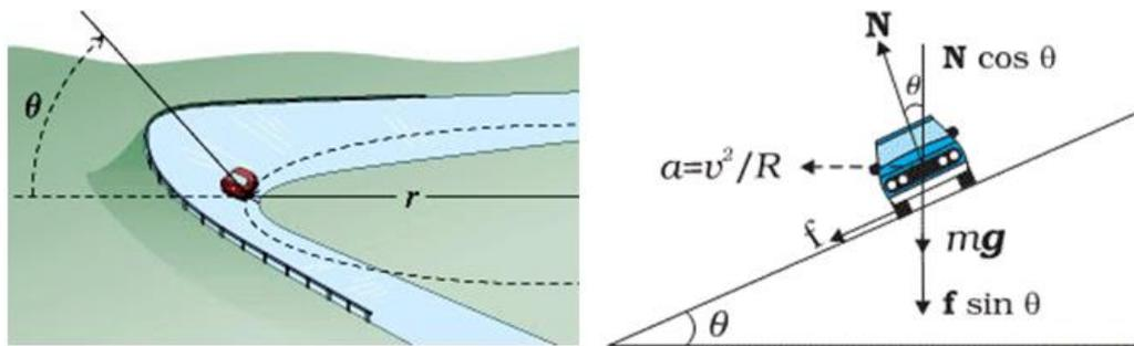
Figure 2 - Basic analysis of cornering forces, see Granlund et al (2014) [9]
