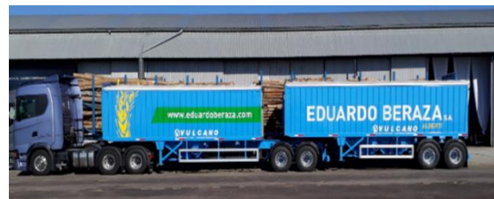
Bulk Grain Hopper, length 22.3m Simulated for a GWT of 57t, in Argentina it is allowed a GWT of 60t
