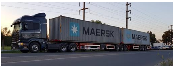
Bitrain with two 40'' containers, length 30.1m Simulated for 71t for Uruguay, in Argentina is allowed a total GWT of 75t.
