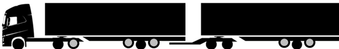
Figure 3 Duo-trailer with five lifted axles
