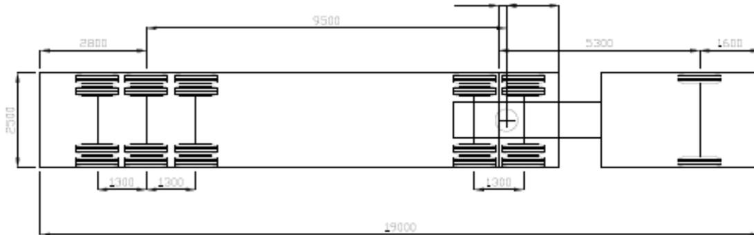
Figure 3. Austroads 19m prime mover and semi-trailer design vehicle.
