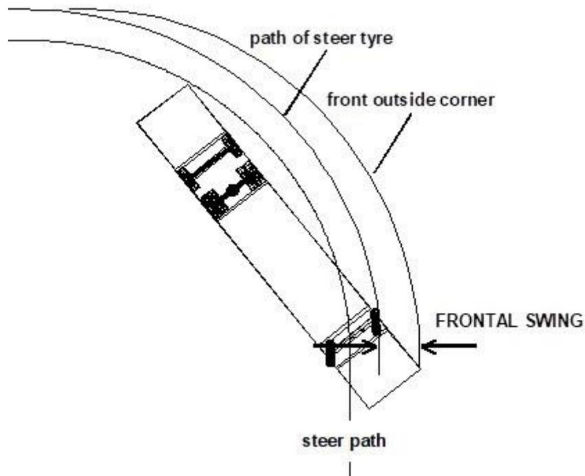
Figure 1. Illustration of frontal swing for a rigid vehicle.
