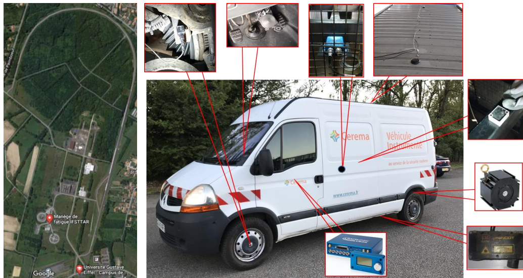
Figure 3: Instrumentation of the Renault Master van
