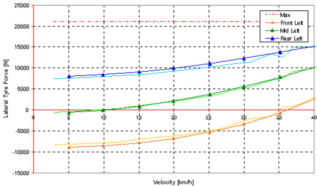
Figure 8. Lateral tyre forces on the three outer trailer tyres, handling test, locked steering.
