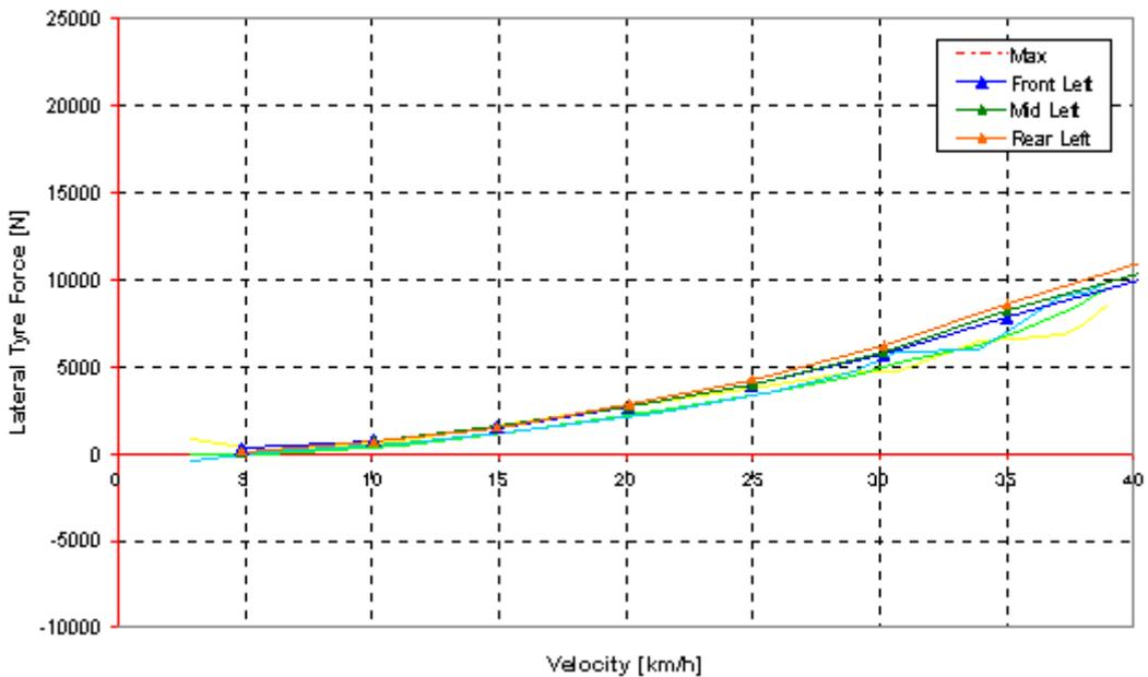
Figure 9. Lateral tyre forces on the three outer trailer tyres, handling test, free steering.
