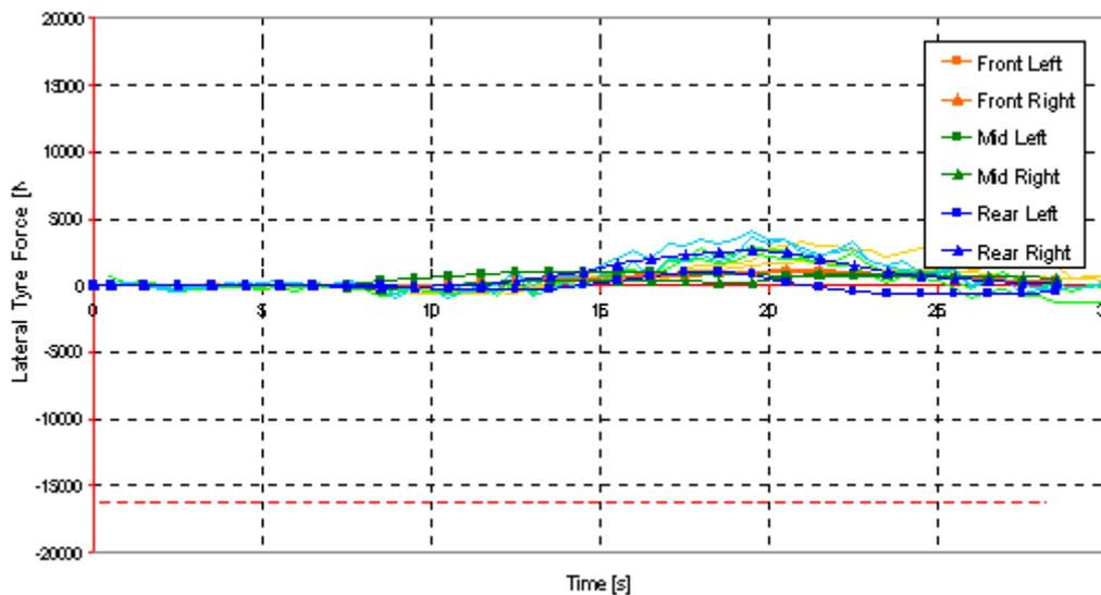
Figure 6. Steering trailer lateral tyre forces- cornering.
