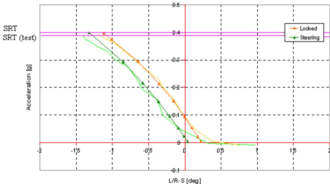
Figure 11. Tractor handling diagram- handling test.
