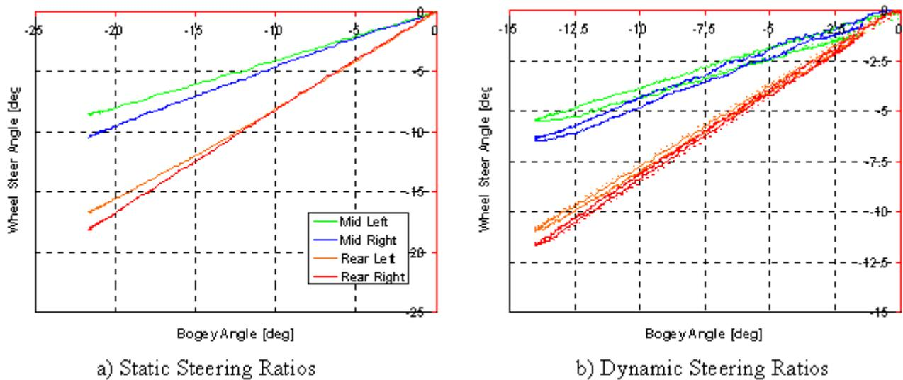
Figure 4. Bogie steering behaviour.
