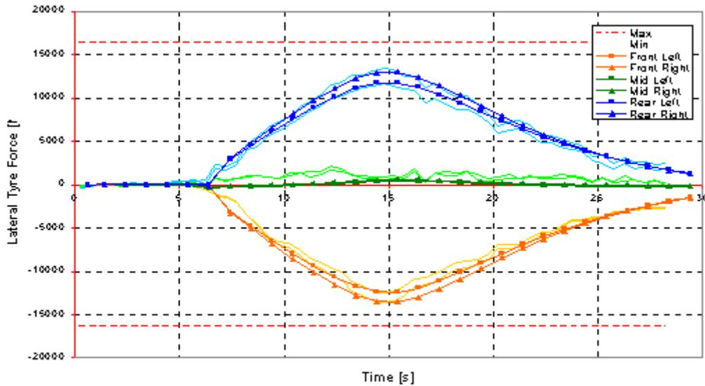
Note: Dashed red lines indicate force generated when the tyre's contact patch is fully sliding
