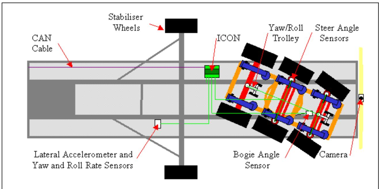
Figure 3. Plan view of trailer unit showing steering bogie and instrumentation.
