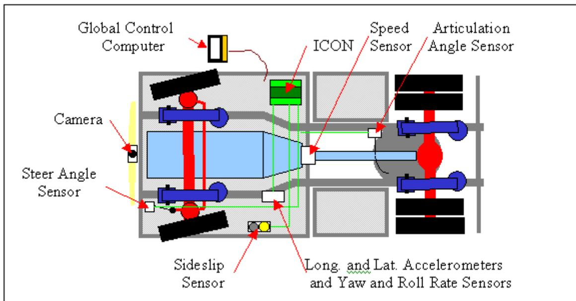
Figure 2. Plan view of tractor unit showing instrumentation.
