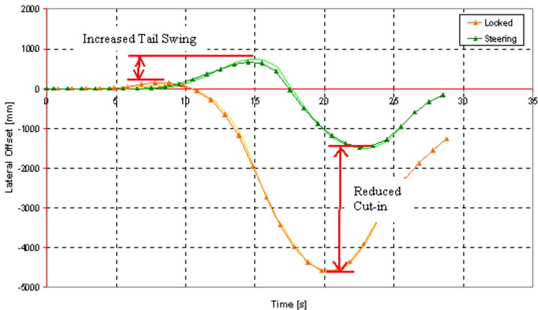
Figure 7. Lateral offset at the rear of the trailer- cornering.
