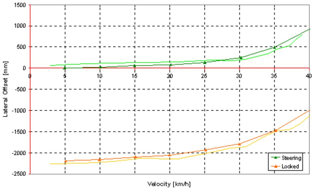
Figure 10. Lateral offset at the rear of the trailer-handling simulation.
