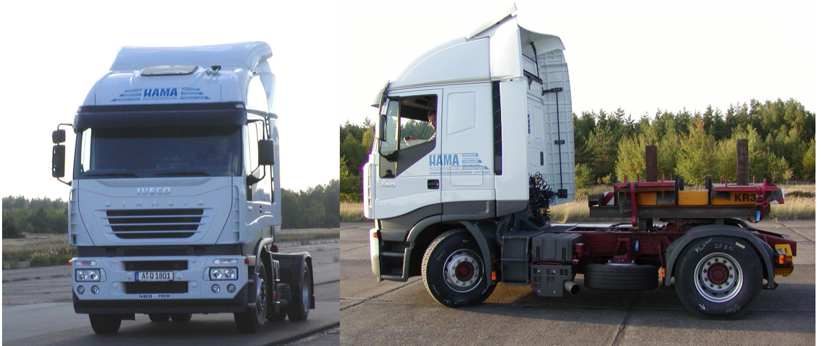
Fig 4: Test Vehicle, Iveco Stralis with Additional Load on the 5 th Wheel
