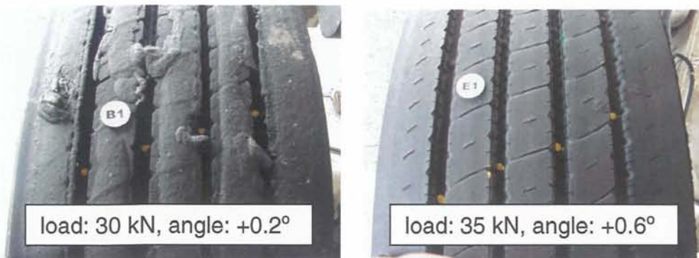
Figure 10 - Truck tyres after carousel tests for different applied loads and slip angles may have become worthless for wear measurements due to clotting of debris (left panel) or have worn in a realistic fashion (right panel).
