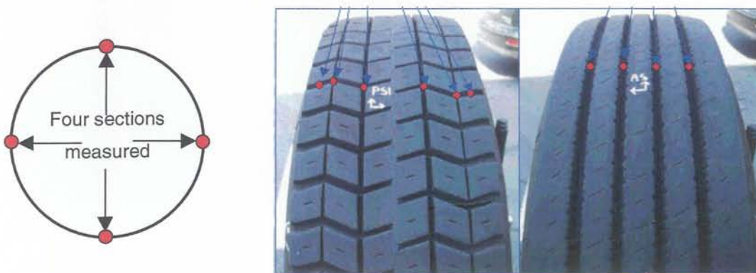
Figure 7 – Truck rear (middle panel) and front tyres (right panel) tread depth were measured at six and four positions across the tyre width, respectively. Tread depth at each position across the tyre were averaged for four positions along the tyre circumference (left panel).
