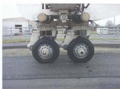
Figure 4 – Carousel test set-up (4 arms of 19 meters long; two truck tyres mounted at each arm).
