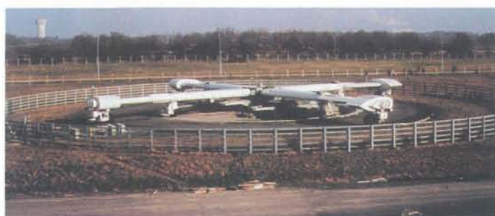
Figure 4 – Carousel test set-up (4 arms of 19 meters long; two truck tyres mounted at each arm).
