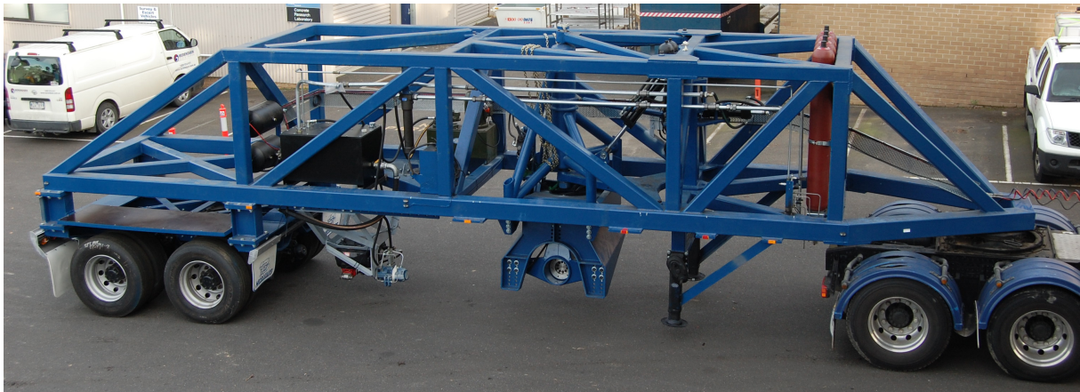
Figure 1 – Tyre force and surface wear mobile rig
