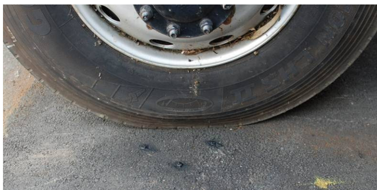
Figure 3 – Test tyre positioned on test section
