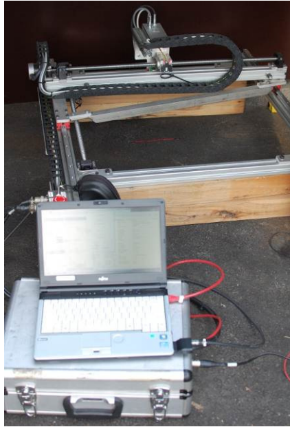
Figure 2 – Surface topography laser rig
