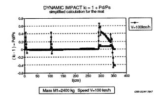
Fig. 3 Theoretical impact effect of the loops and the capacitive mat installed on the pavement surface
