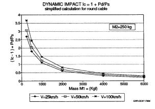
Fig. 2 Theoretical effect of speed at the passage over an obstacle, for different sprung masses
