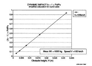
Fig. 1 Theoretical effect of obstacle height on I<sub>e</sub>
