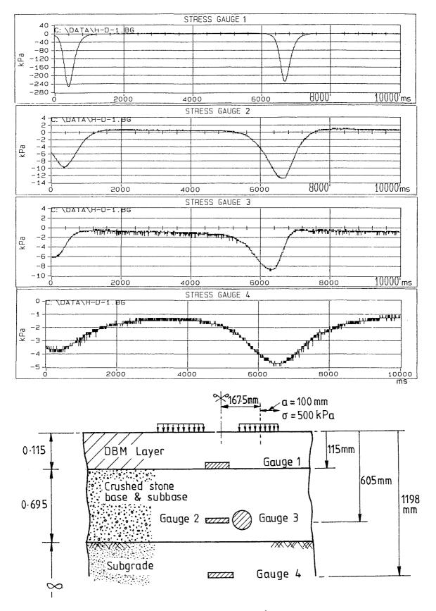
Fig. 3 Stress measurements under Heavy Vehicle
