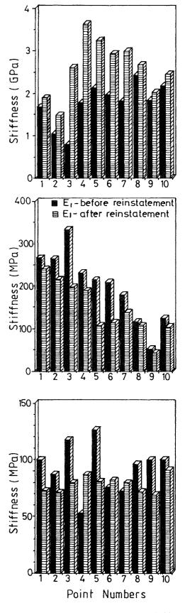
Fig. 2 Changes in Pavement Moduli due to Reinstatement
