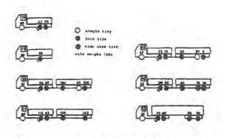
Different trucks and truck combinations used in 1983 FIGURE 6 All the tires were radial ply tires (not bias tires). Special wide base (super single) tires were used instead of ordinary twin tires in types B, G and L. The tire pressures were usually 800 kPa (115 psi), in one case (B) also 700 and 900 kPa (100 and 130 psi) were used.
