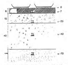
Cross section of a test structure. T2, T5 and T8 are pressure cells, 3 is a strain gage. This measures in centimeters FIGURE 2
