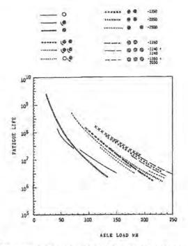
The comparisons of different axles based on the vertical stresses in the subgrade FIGURE 11
