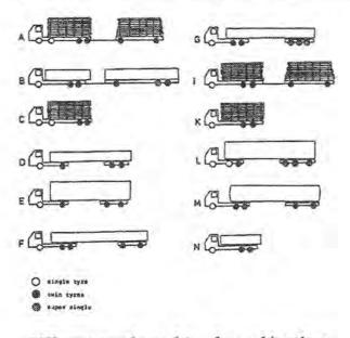
Different trucks and truck combinations used in 1984 FIGURE 7 is in principle the fatigue life of that pavement, that is to say the number of equivalent loads that deteriorates the pavement. The fatigue curves, which were used in making the Shell Pavement Design Manual, were utilized in this study. The basic concept is generally approved and widely used in pavement design.
