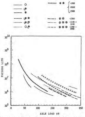
The comparisons of different axles based on the horizontal strains in the asphalt concrete FIGURE 8 The mixed tandem axle is the most detrimental of the driving axles. A tandem axle with both axles driving was the most advantageous.
