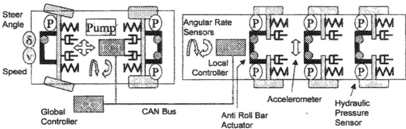
Fig. 6. Sensors, Actuators & Controllers.
