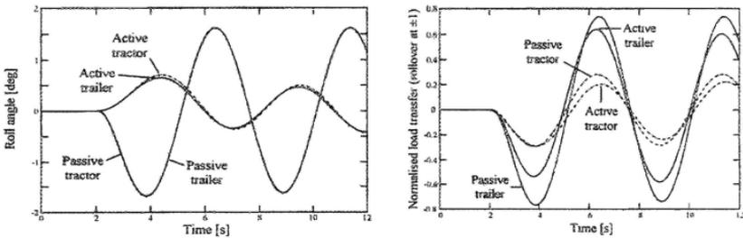
Fig. 5. Response of active and passive vehicles during a lane change manoeuvre: (a) roll angle; (b) load transfer.
