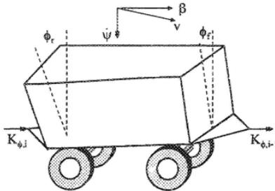
Fig. 2. Schematic diagram of a generic vehicle unit.
