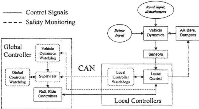
Fig. 3. Schematic of Vehicle and Controller interactions.
