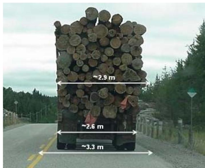
**Figure 3** – Width of Load Exceeds the Allowable Width.
