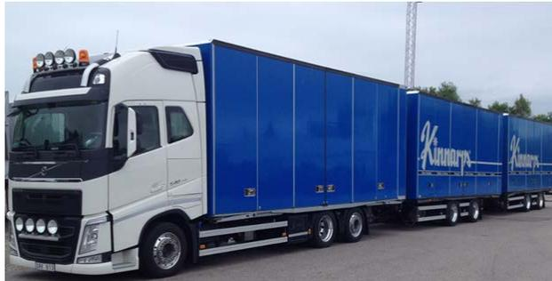
**Figure 3 – A double center axle trailer combination**
