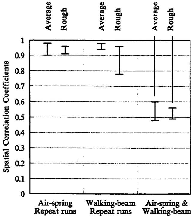
Figure 6. Correlation coefficients between specific wheels from similar and different tractor suspensions.
