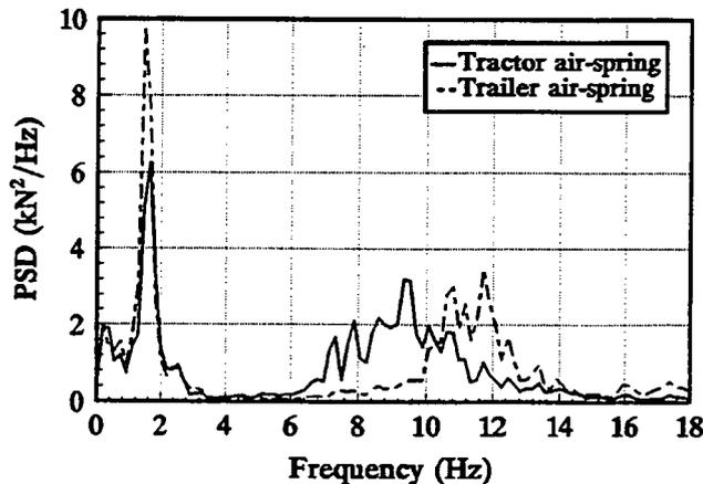
Figure 9. Typical PSDs for tractor and trailer air-spring suspensions.
