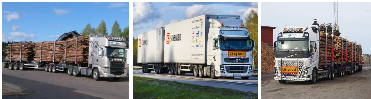
a) Timber truck (GVW 74tonne, length 24m) b) A-double (GVW 80tonne, length 32m) c) ETT vehicle (GVW 90tonne, length 30m)
