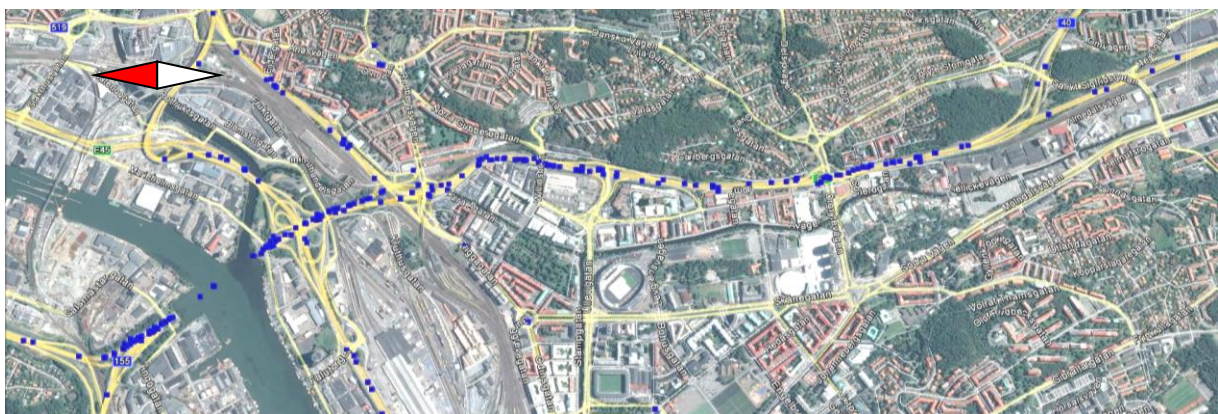
Figure 3.2 – Lane-change crashes (blue dots) on E6 passing through the city of Göteborg, Sweden, involving conventional heavy vehicles 2003-2013 (picture from Google™ Earth).
