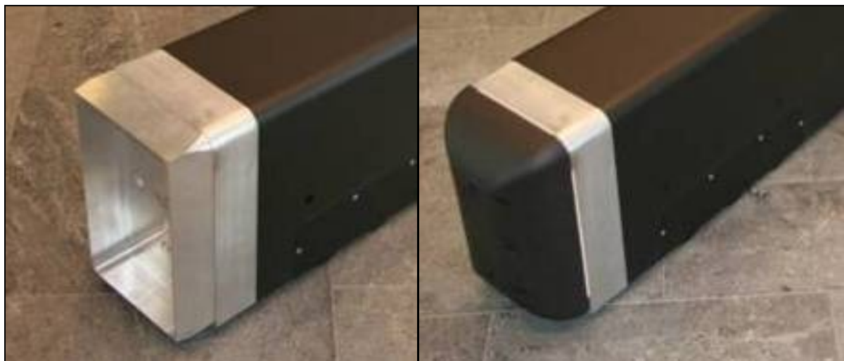
Figure 9. Detailed picture of the boundary-layer blowing units. The left is the one used in the Mod 1 and Mod 3 having 10 degrees angle and the right in Mod 2 having arc with radius of 100mm in the scale model.
