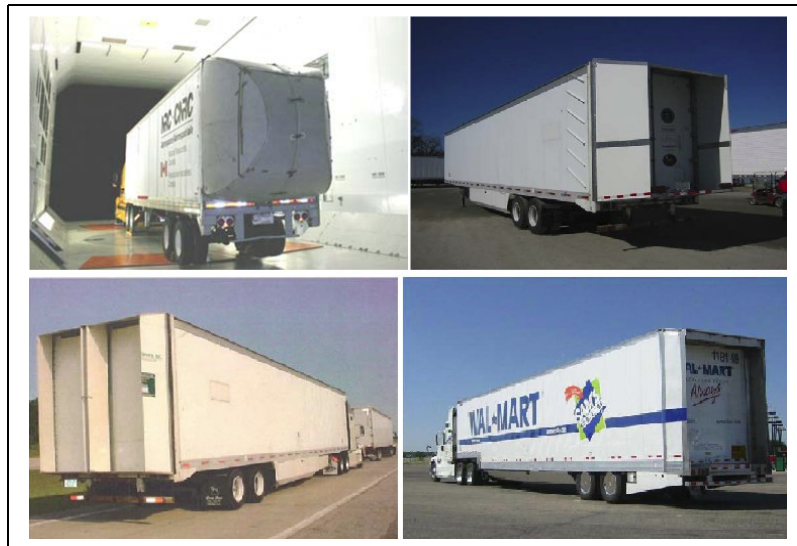
Figure 5. Different boat tail construction in full scale. /Leuschen, TMA/
