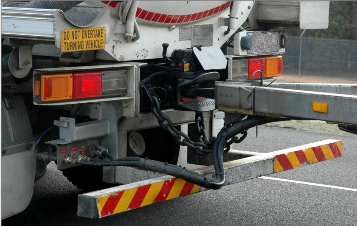
FIGURE 2 – Pin-coupling, release mechanism and safety chain arrangement
