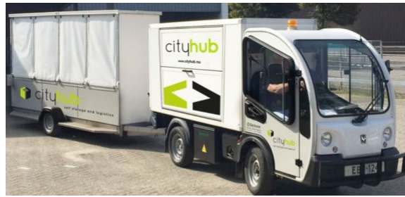
Figure 4: Current situation CityHub, a LEFV tows a trailer with four rolling containers
