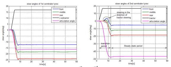
Figure 3. Steering angles of the axles of 1<sup>st</sup> and 2<sup>nd</sup> semi-trailers – Path following strategy
