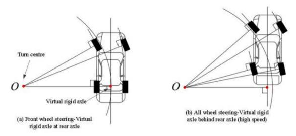
Figure 8: Illustration of virtual rigid axles and turn centre [11].
