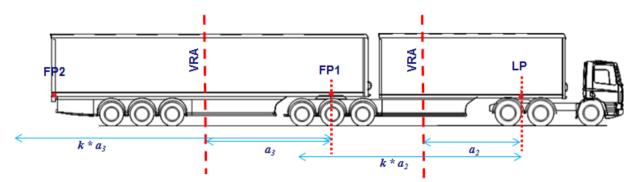
Figure 9: The position of the Virtual Rigid Axle shifted backward at high speeds.
