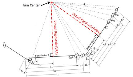
Figure 4: Schematic of a B-double with trailer steering at low speed.
