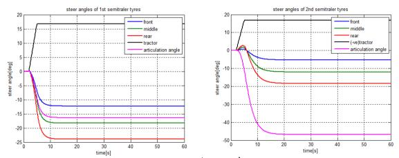
Figure 2. Steering angles of the axles of 1<sup>st</sup> and 2<sup>nd</sup> semi-trailers– Command steering
