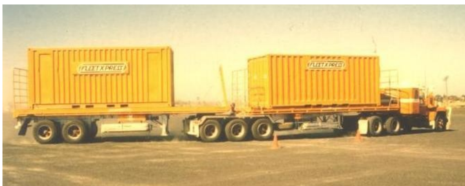
Figure 4: First B-double to use the Canadian concept of triaxle in the middle
