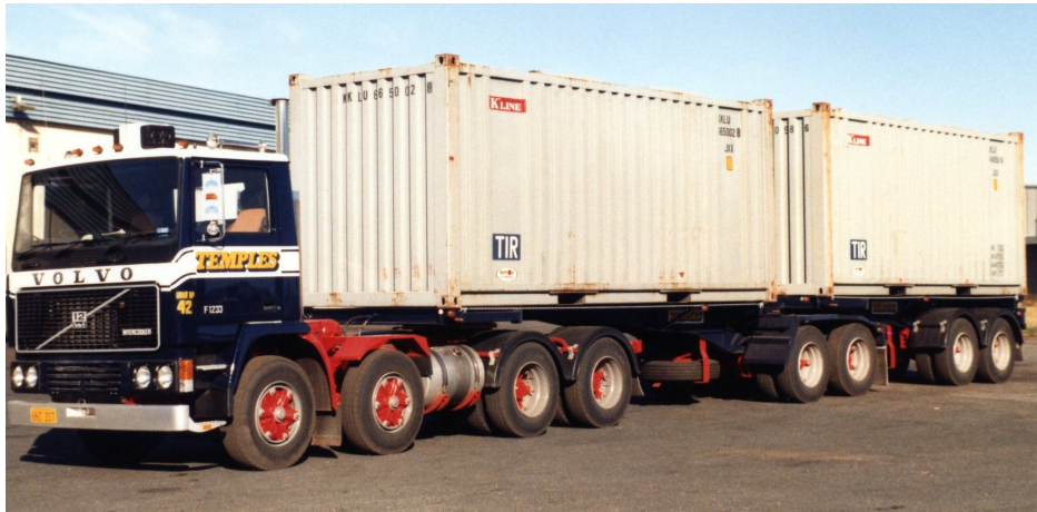
Figure 2: Second Australian B-double at 17 metres long, with tandem axles (incl. steer)
