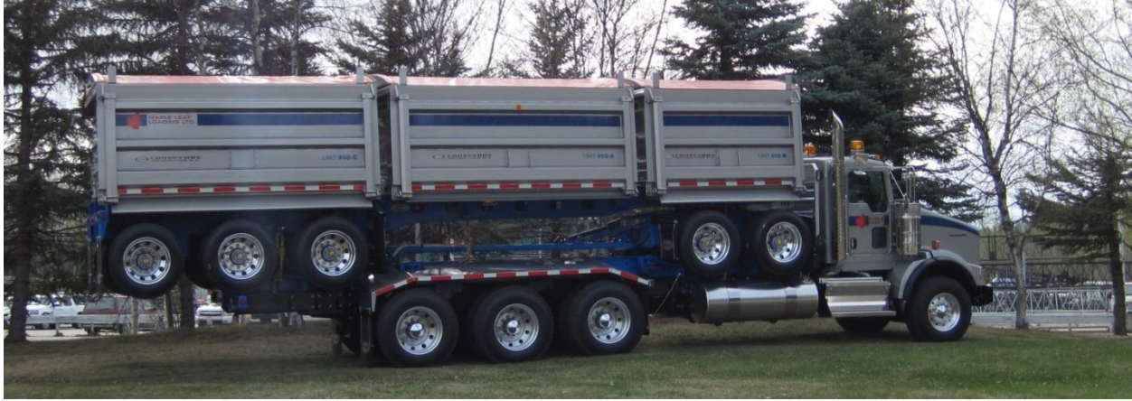
Figure 2. Quint-axle trailer(ore) stacked on truck when empty
