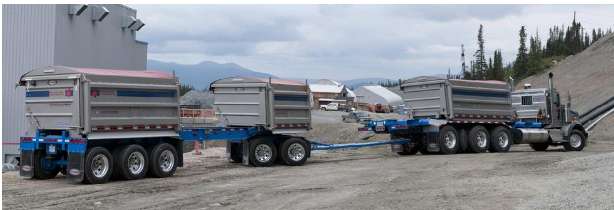
Figure 1 – Tridem truck/ quint-axle full trailer hauling ore
