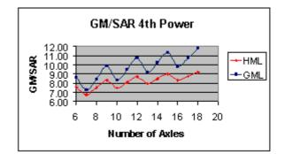
Figure 1. Variation of GM/SAR with Axle Numbers from Representative Vehicles.
