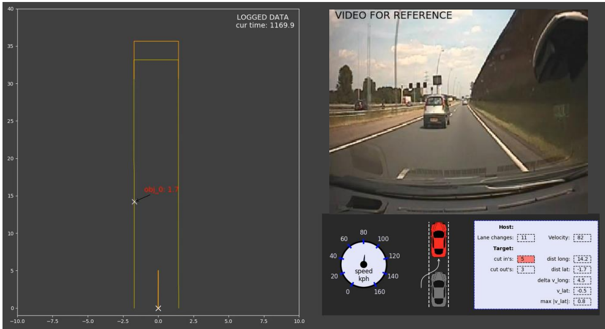
Figure 3: View on a cutting-in vehicle from the data collection vehicle
