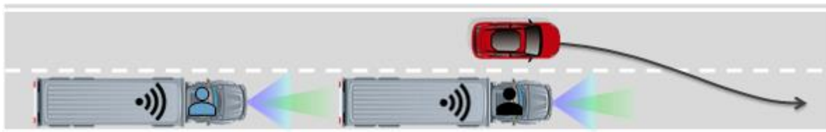
Figure 9: Test case with a vehicle cutting in in front of the platoon.
